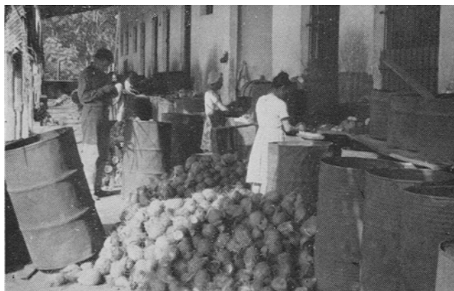
FIG. 5. View in copra shed where the tops of the coconuts are removed to drain the water after which they are split in two and the meat removed for drying.
